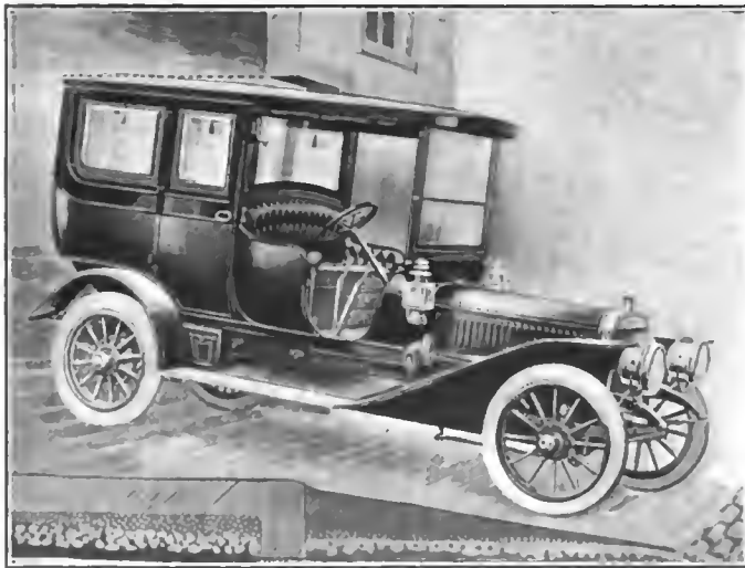
Fig. 1—Showing a limousine passing through the door with the front wheels on the runway and an incline such as will cause the back of the limousine to strike the top of the door framing
